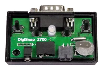
The DigiSnap 2700 has a simplified feature set compared to the other members of the DigiSnap 2000 family, reducing the configuration complexity substantially. The DigiSnap 2700 is intended for use with SLR and other 'contact' style camera interfaces. In addition, a Real-Time Clock has been added, to more easily use the Advanced Time-Lapse feature of the DigiSnap controllers.
