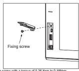
3) Tighten the screw with a torque of 0.36 N•m to 0.48N•n
