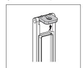
2) Put the provided fixing screw through the hinge hole. Fit the hinge projections of the USB environmental protection cover in the GOT guiding holes and fit the fixing screw of the USB environmental protection cover in the USB environmental protection cover installation hole on the GOT.
