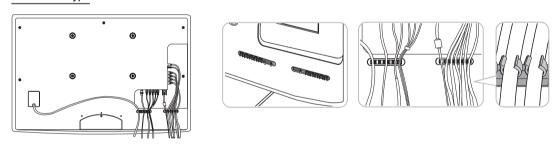
Do not pull the cables too hard when arranging them. This may cause damage to the product's connection terminals.
