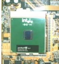
Now with the processor properly installed, you can proceed to install the heatsink. It is important to note that if you have never installed a heatsink on an Intel PIII Tualatin or Coppermine processor before it may be difficult. We recommend you do a dry run a few times before doing the final installation. To allow you to do this read the following instructions. Do not remove the film on the thermally conductive compound until you are ready to do the final installation.
