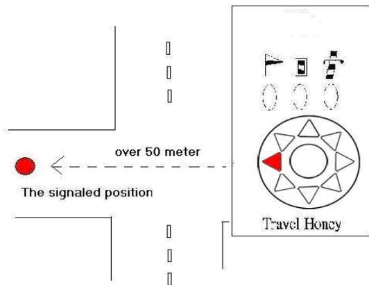
When you are within 15 meters of the destination, the destination (Blue) LED will be on. Following the indication of the direction (Red) LEDs, you can simply find the position saved before.
