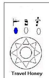
The Destination (Blue) LED flashes after all direction (Red) LEDs have flashed, which indicates the position has been saved. When its at LF mode the device do not store or track any logs, therefore, please switch device DL mode for data log. DL mode can also be used as LF lock key; to prevent destination stored in LF been erased.
