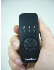
Press the setting button for 2 seconds, and then all direction (Red) LEDs will flash together for 3 seconds.
