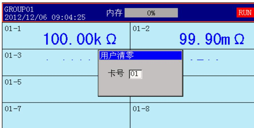
For accurate measurements, zero-adjustment needs to be performed before measurement.
