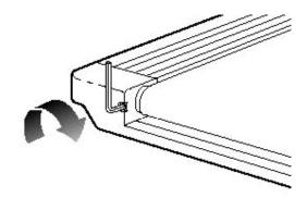
If the walking belt has shifted to the right, first remove the safety key and unplug the power cord. Using the Allen wrench, turn the left adjustment bolt counter-clockwise 1/4 of a turn. Plug in the power cord, insert the safety key, and run the treadmill for a few minutes. Repeat until the walking belt is centered.
