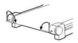
If the walking belt has shifted to the right, first remove the safety key and unplug the power cord. Using the Allen wrench, turn the left rear roller adjustment bolt counterclockwise, and the right bolt clockwise, 1/4 of a turn each. Be careful not to over tighten the walking belt. Plug in the power cord, insert the safety key, and run the treadmill for a few minutes. Repeat until the belt is centered.
