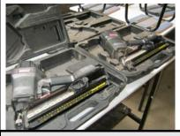
**Potential Hazards:** Discharged nails and pressurised air with the potential to cause harm through direct nail projectiles and indirect ricochets.
