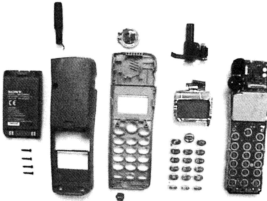
Parts on the main board specified in the parts list can now be reached.
