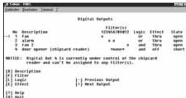
The menu points **[D]**, **[F]**, **[L]** and **[E]** are disabled for DIGITAL OUT 4 whilst, the current status of the output is displayed in the column headed "State".
