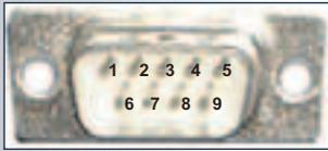
– Serial interface – directly connected to the COM connection on the front of the device.
