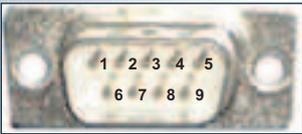
– Serial interface for the connection of external devices (for example, UPS, fans, airconditioners, chipcard reader heating, ...)
