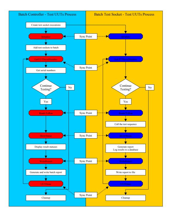
At each sync point in the diagram above, the controlling and test socket executions wait for each other until all are at the same sync point. When they all arrive at the same sync point, the controlling sequence executes its code first, then, before reaching the next sync point, tells the test socket executions to continue executing their code.
