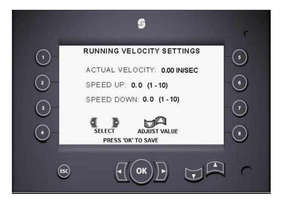
Left and Right Arrow Button will select the setting to adjust. Up and Down Arrow Button will adjust the selected setting. OK Button will save the setting value.
