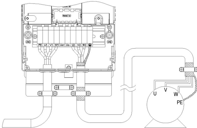
Figure 20 Motor cable connection for frame sizes R3 and R4 (IP 21 / NEMA1).
