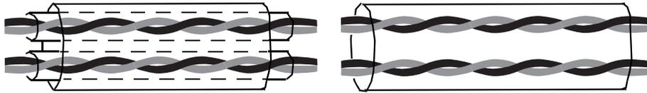
Figure 80 A double shielded twisted pair cable on the left and a single shielded twisted multipair cable on the right.
