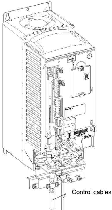
Figure 22 Control cable connections (IP 21 / NEMA1).
