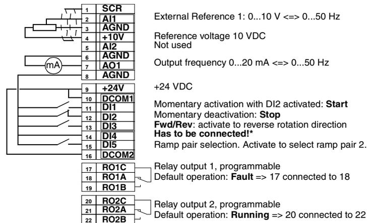
**\*Note!** DI 4 is used to configure ACS 400. It is read only once when power is connected. All parameters marked with \* are determined by the DI4 input.
