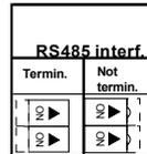
Signal termination is selected with DIP switch.
