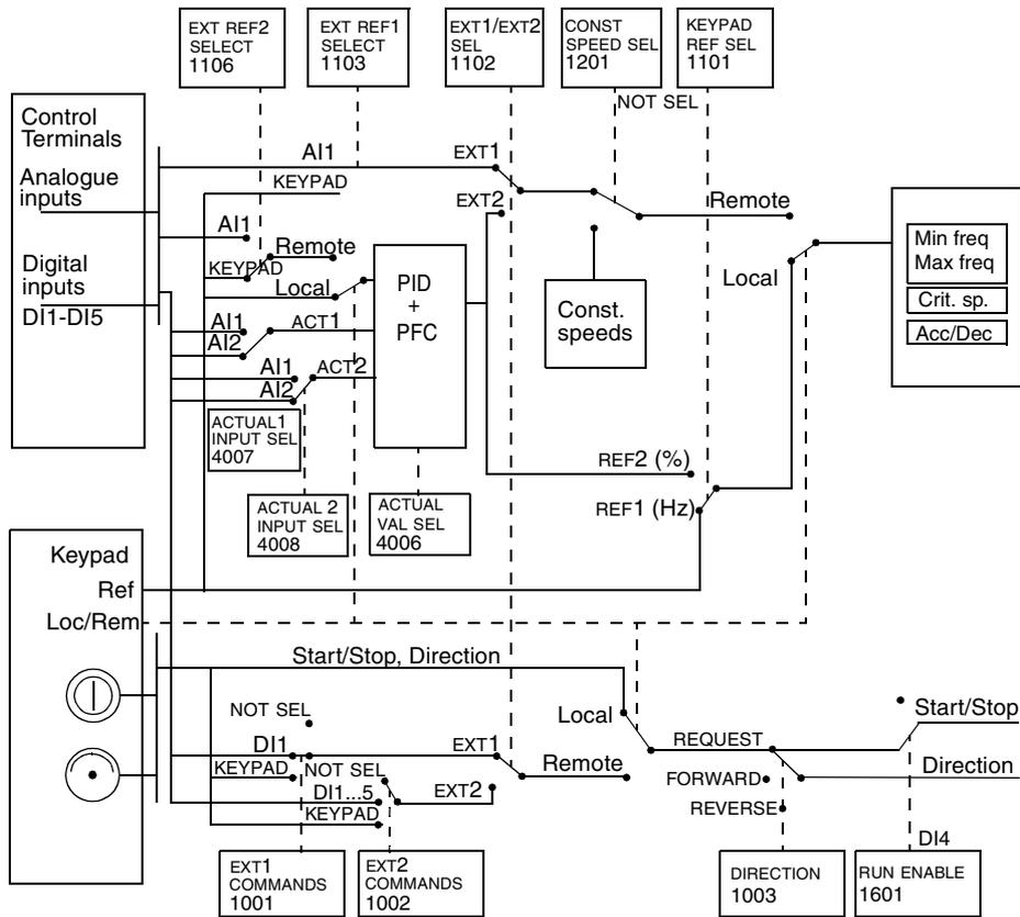
Figure 76 The control signal connections of the Pump and Fan Control (PFC) macro.
