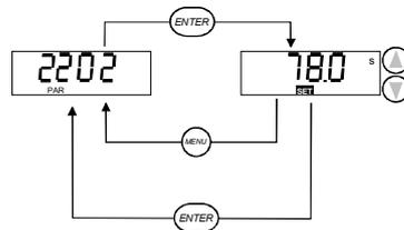
**Note!** **SET** blinks, if the parameter value is altered. **SET** is not displayed, if the value cannot be altered.
