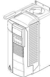
Figure 6 Affixing type IP 21 / NEMA1 frequency converters.
