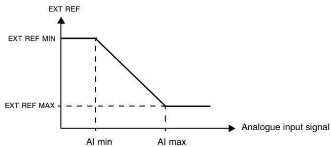
Figure 38 Setting EXT REF MINIMUM and EXT REF MAXIMUM. The range of the analogue input signal is set by parameters 1301 and 1302 or parameters 1304 and 1305, depending on the analogue input used.
