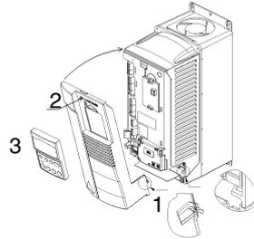
Replacing the front cover to IP 21/ NEMA1 units from size ACS401-x016-3-x and up.
