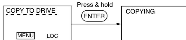
**Note!** Drive must be stopped and in local control. Parameter 1602 PARAMETER LOCK must be set to 1 (OPEN).
