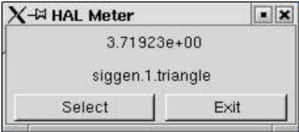
Figure 4.3: Halmeter displaying the value of a pin
