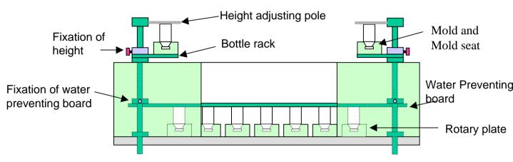
Put a set of mold (including the seat) together with bottle on the bottle rack (1 set for each side), adjust the height adjusting pole to fit the bottles, then put down the fixation of height and lock.
