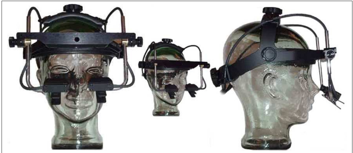
Figure 1.2: The EyeLink II Headset used for eyetracking data collection.
