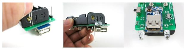
There is a separate LED on/off switch. The 5V/3.3V voltage selector is also effective: at 5V output voltage, the LEDs are considerably brighter than 3.3V, so this can be used for brightness control.
