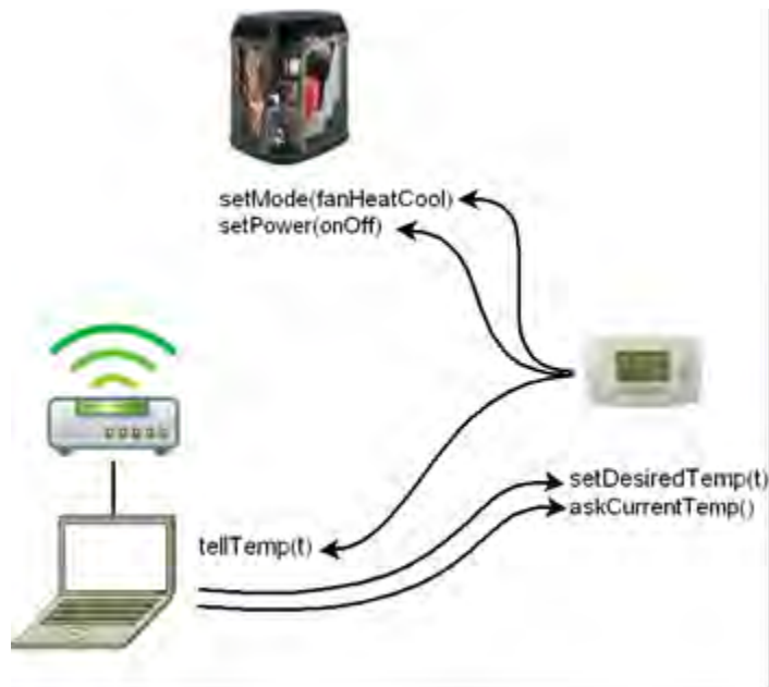
Figure 1 - Example HVAC System Showing RPC Call-flow (arrows)
