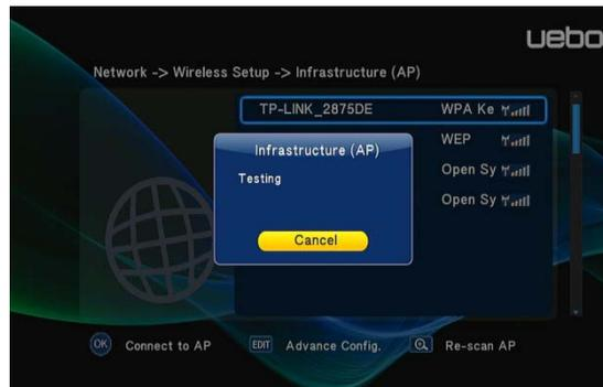
The testing process can take a couple minutes to establish a connection. If the test is ok, the network information (Profile Name, IP address, Subnet Mask, Gateway, etc.) will be displayed on the screen.
