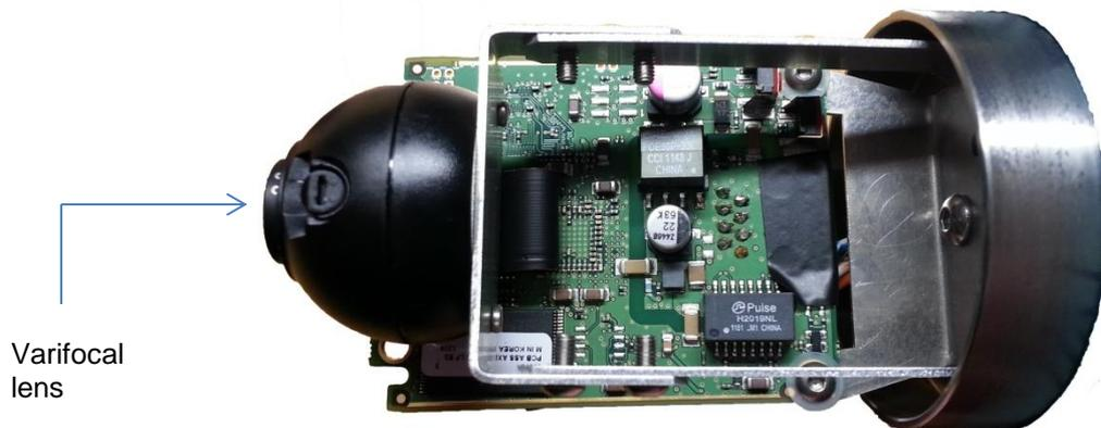
Figure 4.9 Lens and circuit board of the ToughCam IP
