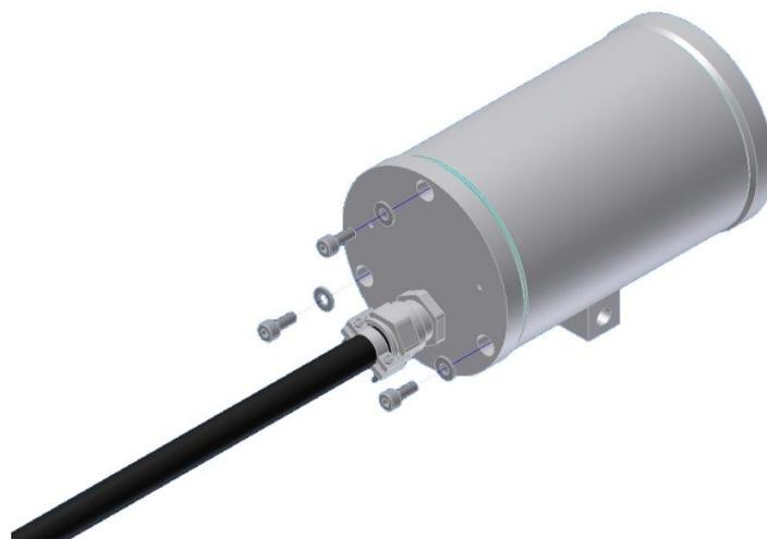
Figure 4.6 Opening of the stainless steel housing (1)
