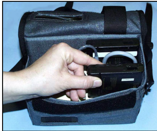
Figure 5-4 VADPAK Battery Bays
