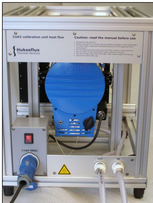
Figure 11.3.1 Picture of calibration unit CU02, showing water supply (in / out), power supply and heat source (1250 Watt lamp, housing in blue). At the background the water-cooled plate on which the sensors are mounted, is visible
