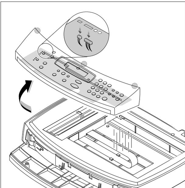
9. Unlatch the Scan Upper securing the Scan Ass'y. Then pull the Scan Upper upward and remove it.
