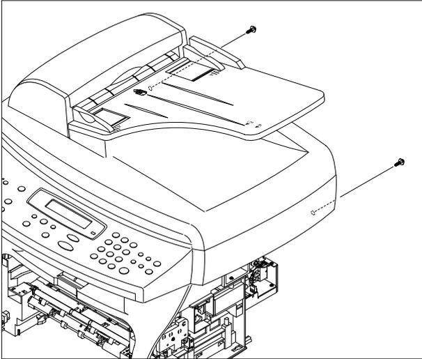
4. Pull up the Scanner Ass'y, as shown below.
