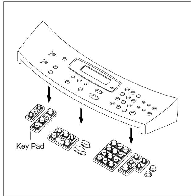
3. Remove the Contact Rubber from the OPE Cover.
