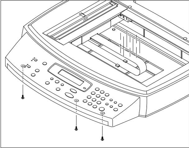
8. Remove the four screws securing the Scan Upper.
