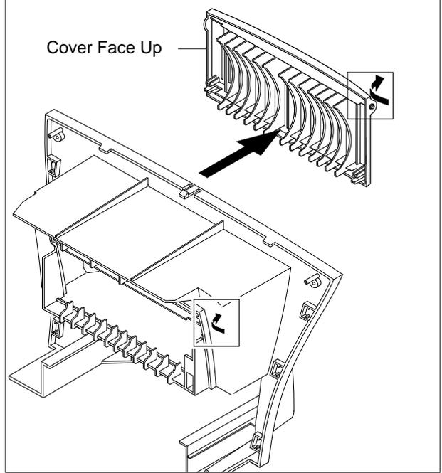
2. Remove the Rear Cover from the Frame Ass'y and Scanner Ass'y.
