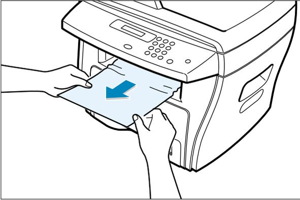
3) If there is any resistance when you pull the paper or the paper is not seen in the front output tray, open the rear cover.
