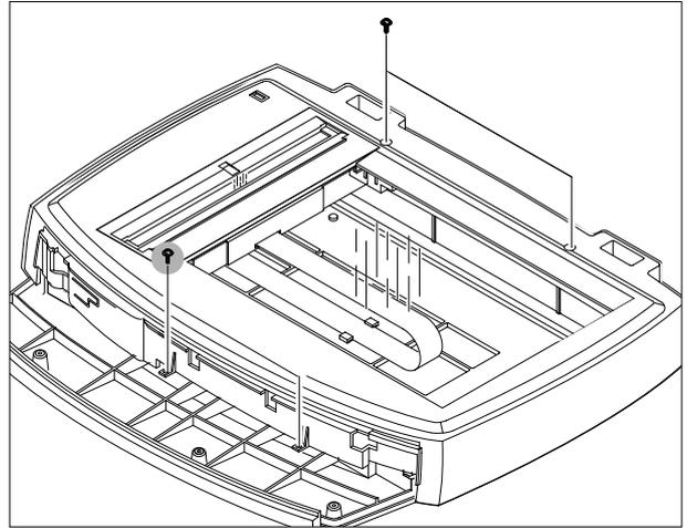
7. Lift the OPE Unit out. Then unplug the two connectors from the OPE Unit and remove it.
