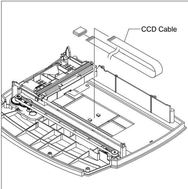
12. Pull up the CCD Shaft and take out the Scanner Module.
