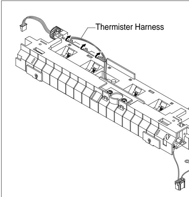
8. Remove the one screw securing the Thermister and remove it, as shown below.
