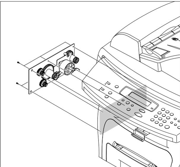
3. Take out the Drive Ass'y, then unplug the connector from the Main PBA, as shown below.
