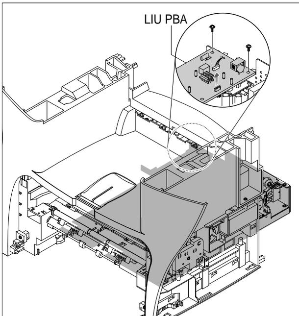
2. Remove the ten screws securing the Engine Shield Ass'y and remove it. Then unplug the all the connectors from the Main PBA and SMPS.
