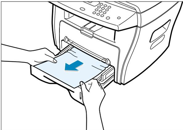
If there is any resistance when you pull the paper or the paper is not seen in this area, skip to the fuser area around the toner cartridge
