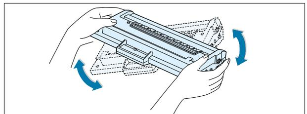
4. Save the box and the cover for shipping. Slide the new toner cartridge in until it locks into place.
