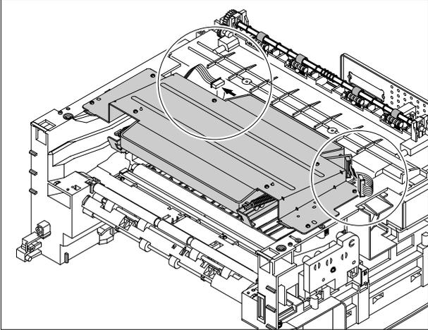
3. Remove the four screws securing the LSU and remove it.
