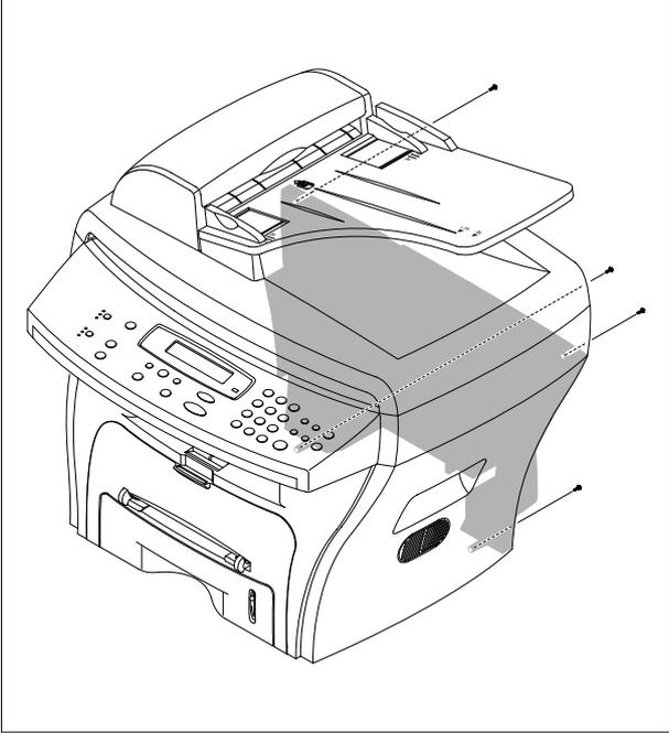
3. Unlatch the (Cover Face Up) securing the Rear cover, as shown below. Then lift the (Cover Face Up) out.
