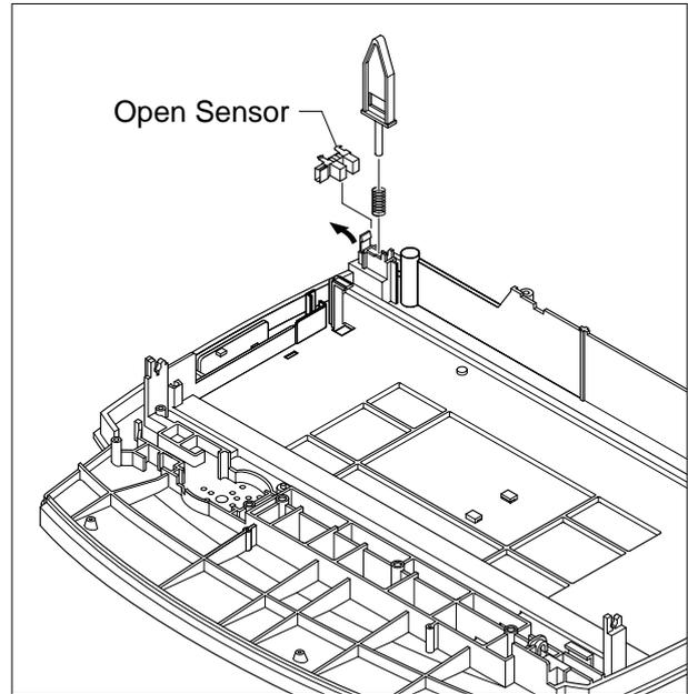
15. Unplug the one connector from the Open Sensor Ass'y.
