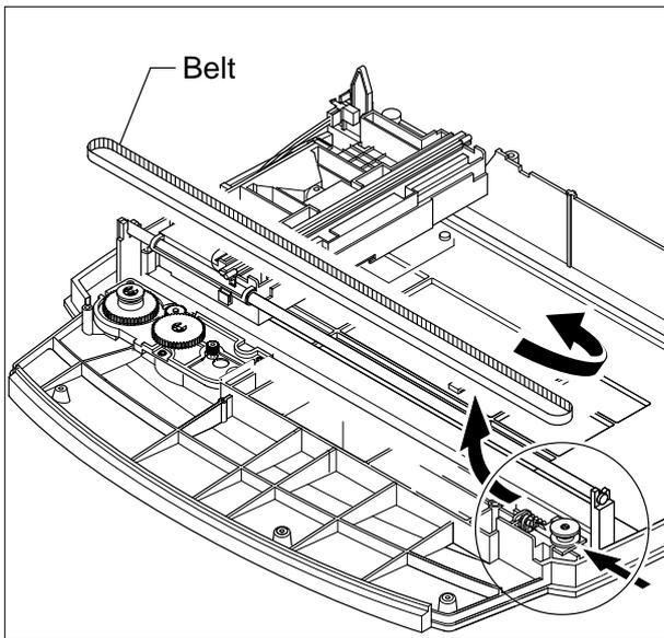
13. Remove the Reduction Gear and Idle Gear, as shown below.
