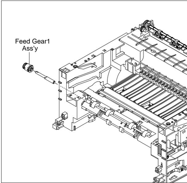
7. Pull up the Feed Roller and Feed Roller1.
