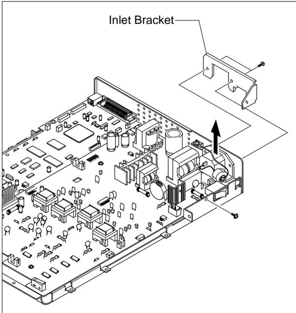
4. Remove the three screws securing the SMPS. Then lift the SMPS out, as shown below.
