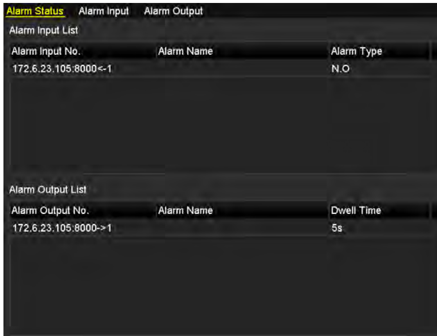
Figure 8. 4 Alarm Status Interface of System Configuration
