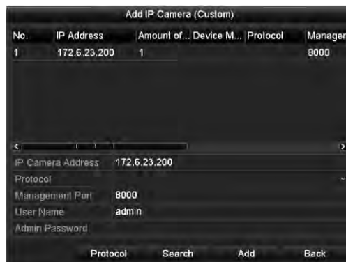
Figure 2. 14 Custom Adding IP Camera Interface
