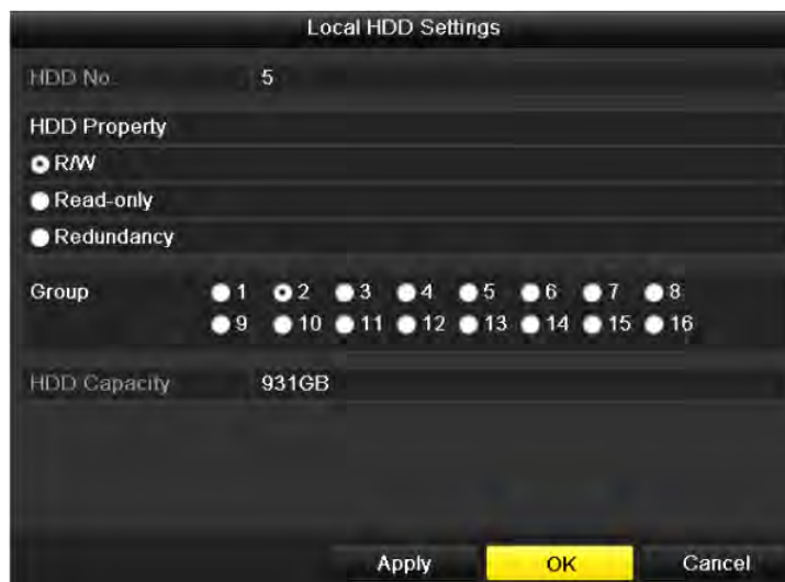
Figure 10. 12 Local HDD Settings Interface
