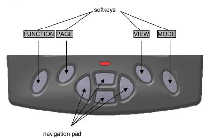
Centre keys are a 'navigation pad' ( UP DOWN LEFT RIGHT ). Softkeys are situated on either side of the navigation pad. The current function is shown on the soft-key menu area at the bottom of the LCD. The MODE softkey switches between the three operating 'modes' (NAVTEX, Navigate & Setup).
