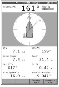
the usual meteorological wind symbol rules: 5kts per half feather, 10kts per full feather, 50kts per triangle. Computed Set and Drift and other related parameters are shown in digital form at the bottom of the screen.
