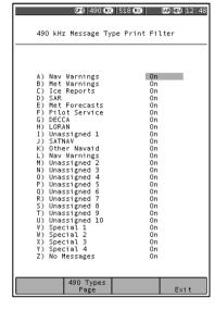
to your current position, set the auto station filter to Nearest. To print messages from all stations in range of your current position, set the auto station filter to In Range. An asterisk appears next to all stations for which messages will be printed.
