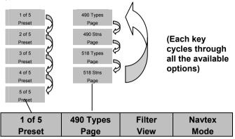
Pressing the PRESET softkey changes the active preset number. The filter page settings change as each different preset number is selected. Similarly, the PAGE softkey changes the filter pages applicable to the selected preset.
