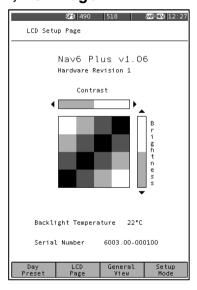
If 'Night Preset' is visible in the softkey menu area then the contrast and brightness control bars show the current 'Night' settings. These can be changed using the <a href="LEFT">LEFT</a>, <a href="RIGHT">RIGHT</a>, <a href="UP">UP</a> and <a href="DOWN">DOWN</a> keys.
