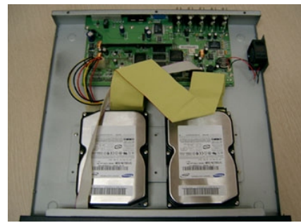
Two HDD Installation
