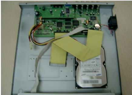
One HDD Installation
