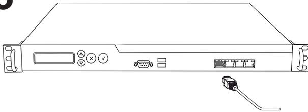
Connect the Ethernet LAN cable to socket LAN 1.
