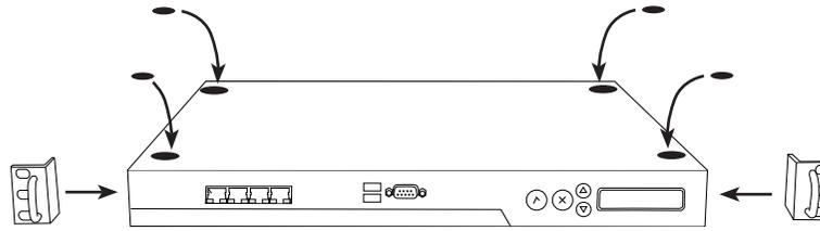
Mount the rack ears and/or rubber feet, if applicable, and turn the unit back on its feet or mount it in the rack.
