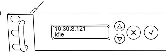
The Content Server will be assigned an IP address from a DHCP server in the network. The automatically assigned IP address will be visible in the display shortly after power up, e.g. 10.30.8.121.
