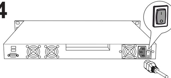
Connect the power cable and turn on the unit.
