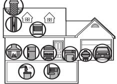
Fuel-burning appliances like: portable heater, gas or wood burning fireplace gas kitchen range or cooktop, gas clothes dryei Damaged or insufficient venting: corroded or disconnected water heater vent pipe, leaking chimney pipe or flue, or cracked heat exchanger, blocked
