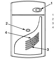
Test/Silence Button POWER/ALARM Light (Red) 3 Air Vents 4 Alarm Horn: 85 dB audible alarm for test, alarm, and unit
