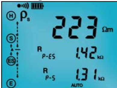
The Schlumberger test displays test lead connection, soil resistivity (ρ) test results, test electrode resistance and more.
