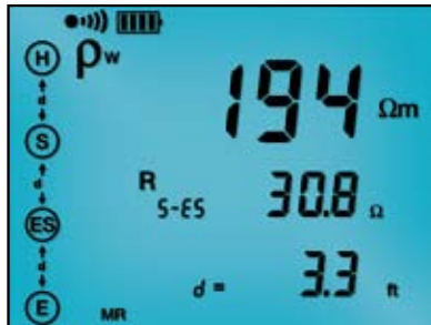
The Wenner test displays test lead connection, soil resistivity (ρ) test results, electrode spacing and resistance.
