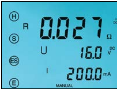
The 4-Point Bond test shows lead connections, bond resistance test results, test voltage and current.
