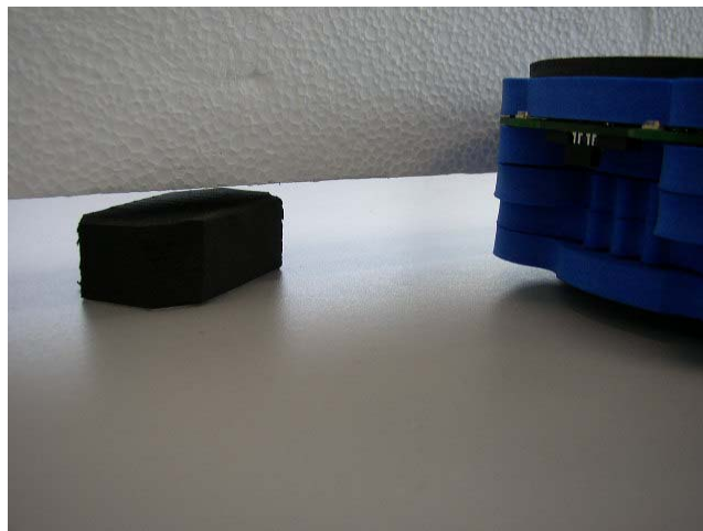
Figure 121: Foam block under the arena wall with Hemisson IR detecting the wall
