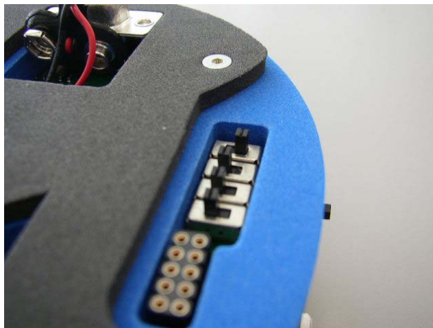
Figure 22: Run and Download user program mode switch setting
