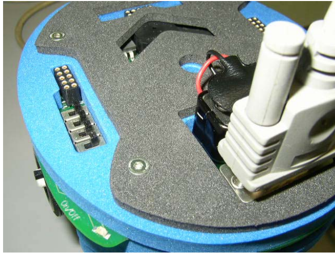
Figure 23: Serial port and TV remote mode switch settings
