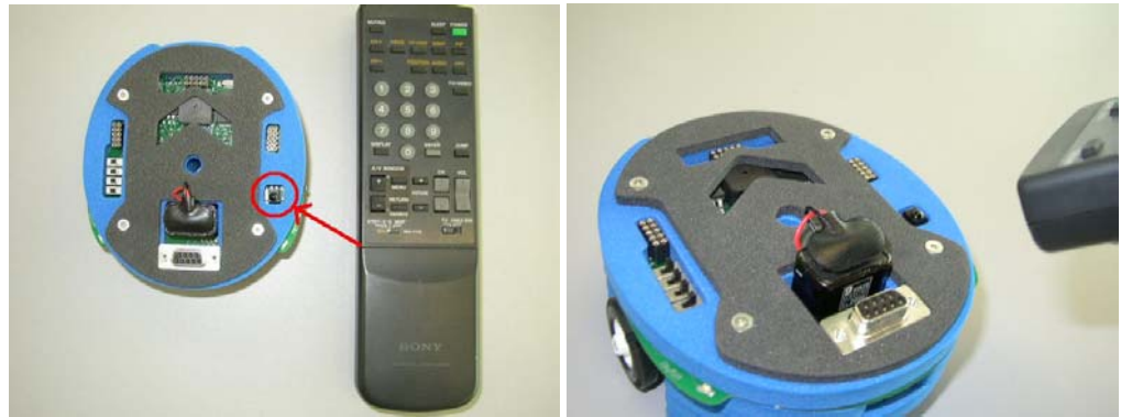
Figure 29: Location of IR receiver for TV remote and Hemisson being controlled by TV remote
