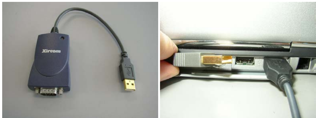
Figure 26: USB to Serial port Adapter and USB port shown on back of Notebook computer
