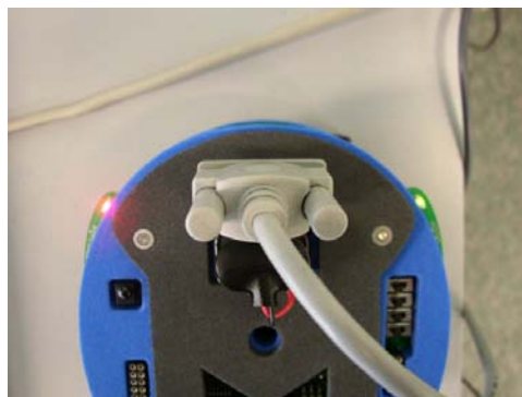
Figure 58: Red and Green LED are solidly lit up when in Pgm mode
