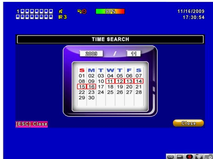
Click 'date' to display the recording times of that specific date with a time bar. You can change time (hour/minute/second) or click on a specific time within the time bar using the mouse then pressing OK. The DVR will playback the selected recorded data.
