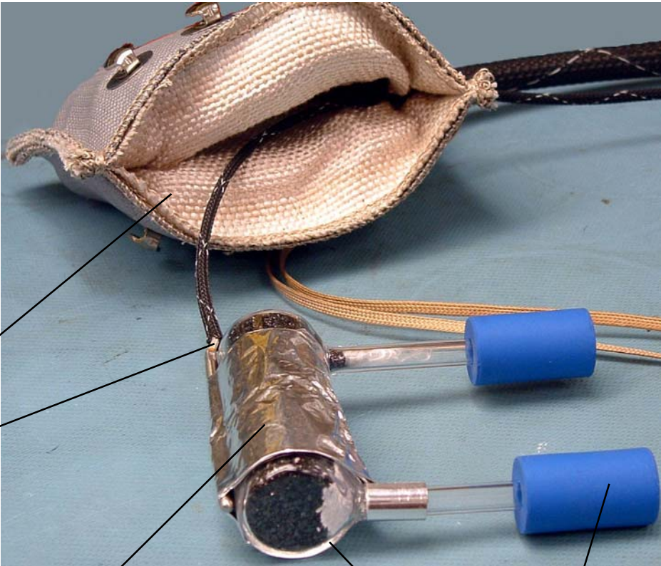
Wrap with Aluminium Foil Converter Tube (655227) Connectors (632784)
