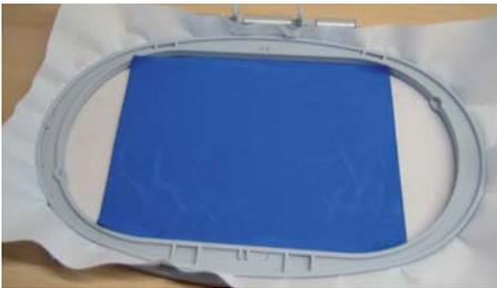
2. Attach foam rubber with temporary adhesive.
