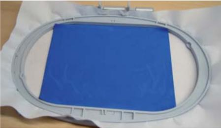
3. Insert CutWork Tool in sewing computer and cut out motif according to sewing computer instructions.
