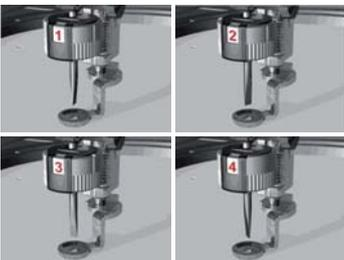
The cutting line in a CutWork design is split up and indicated in 4 different colours. The colours refer to the 4 positions of the BERNINA CutWork Tool.
