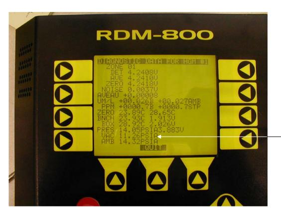
Observe "PRES", "VAC" and "AMB" readings during the check procedure
