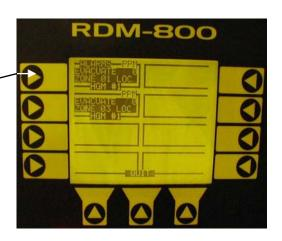
STEP #4: PRESS THIS BUTTON TO ACKNOWLEDGE THIS ALARM. ANY OTHER ALARMS WILL HAVE TO BE DEALT WITH IN THIS WAY TO SHUT OFF THE ALARM HORN!
