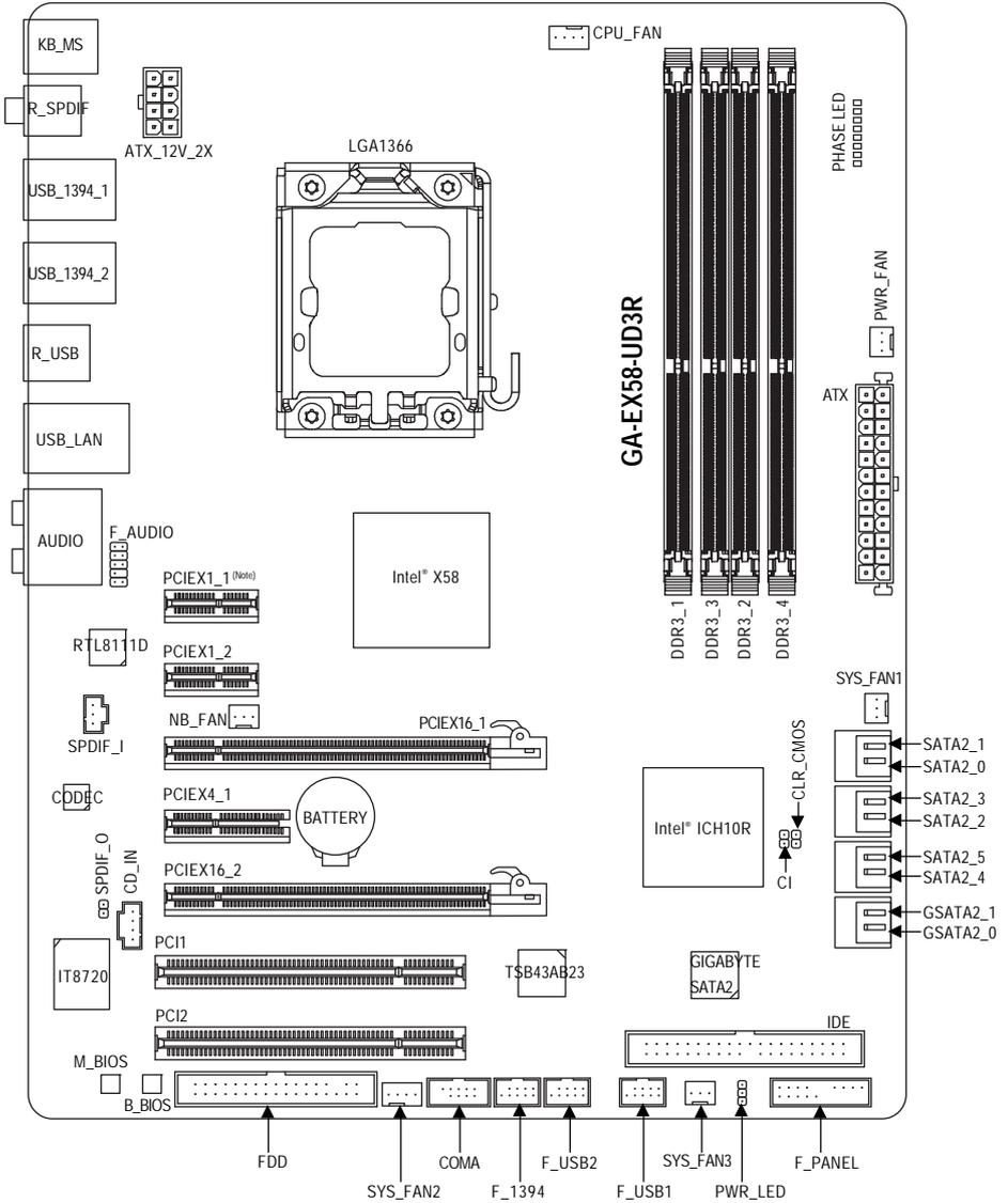
(Note) Due to a hardware limitation, the PCIEX1\_1 slot can only accommodate a shorter PCI Express x1 expansion card. For a longer expansion card, use other expansion slots.
