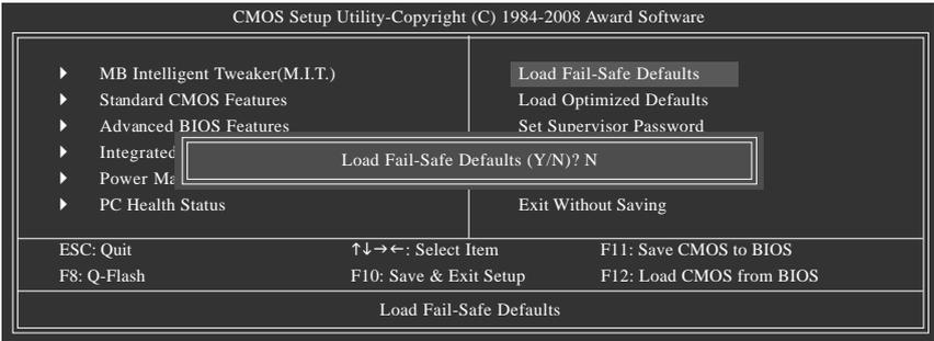
Press <Enter> on this item and then press the <Y> key to load the safest BIOS default settings. In case system instability occurs, you may try to load Fail-Safe defaults, which are the safest and most stable BIOS settings for the motherboard.
