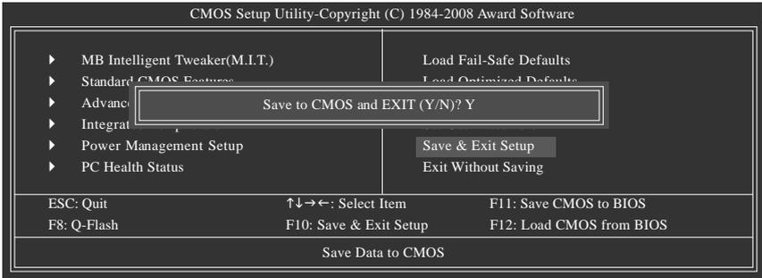
Press <Enter> on this item and press the <Y> key. This saves the changes to the CMOS and exits the BIOS Setup program. Press <N> or <Esc> to return to the BIOS Setup Main Menu.
