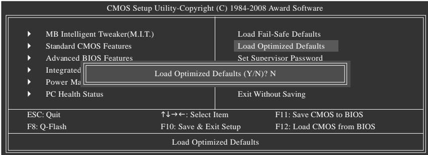
Press <Enter> on this item and then press the <Y> key to load the optimal BIOS default settings. The BIOS defaults settings helps the system to operate in optimum state. Always load the Optimized defaults after updating the BIOS or after clearing the CMOS values.
