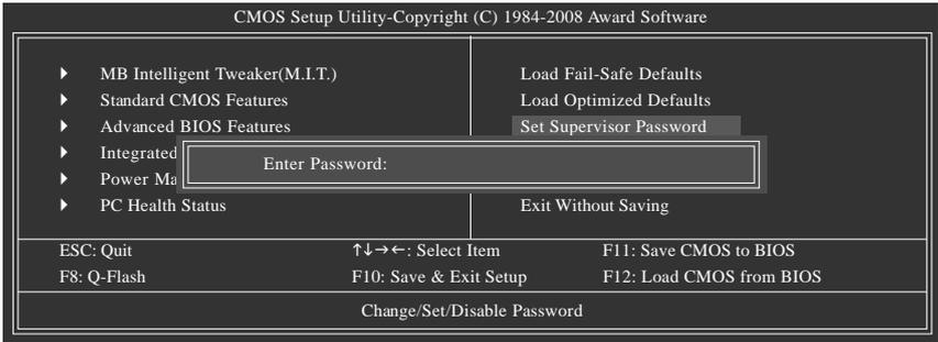
Press <Enter> on this item and type the password with up to 8 characters and then press <Enter>. You will be requested to confirm the password. Type the password again and press <Enter>.
