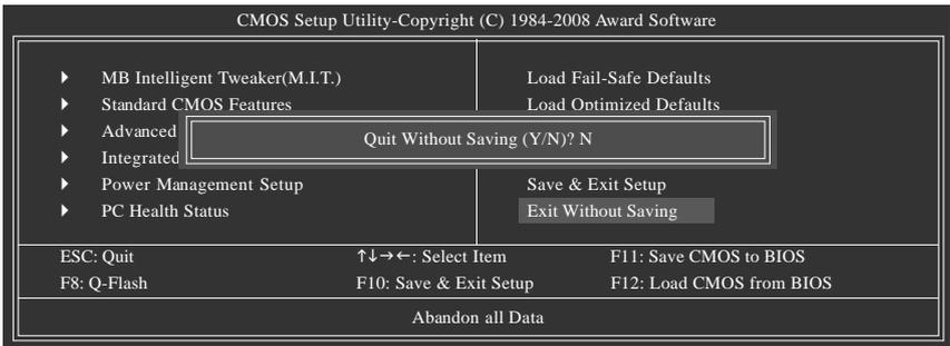
Press <Enter> on this item and press the <Y> key. This exits the BIOS Setup without saving the changes made in BIOS Setup to the CMOS. Press <N> or <Esc> to return to the BIOS Setup Main Menu.
