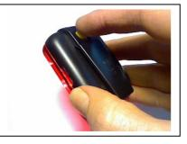
Whenever the tracker detects movement, it will begin uploading its location to the GPSTrackThis website at regular intervals. It will do this until 5 minutes after the vibrations stop
