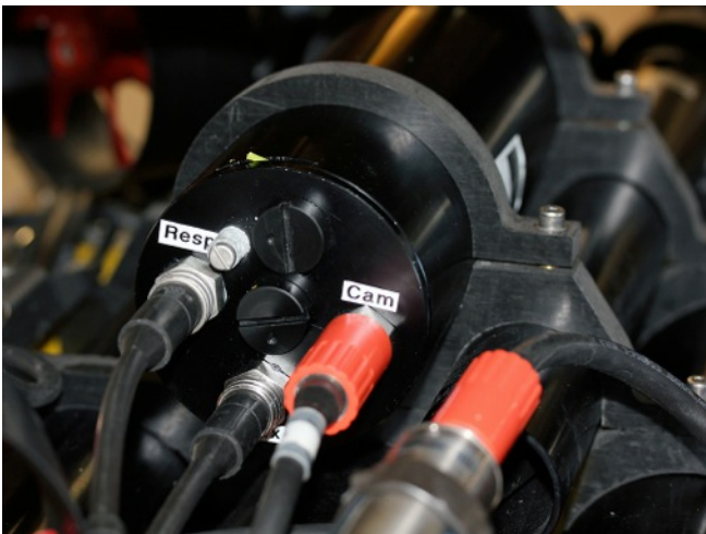
Interface connectors on permanently terminated FT
