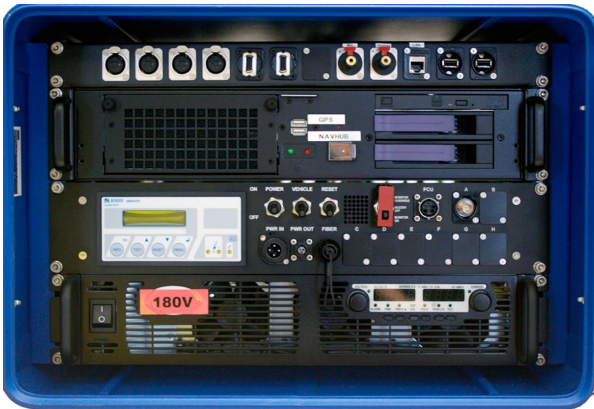
A typical SU for a fiber-optic umbilical V4 system in an aluminium mobile case containing a PU, SIU and computer
