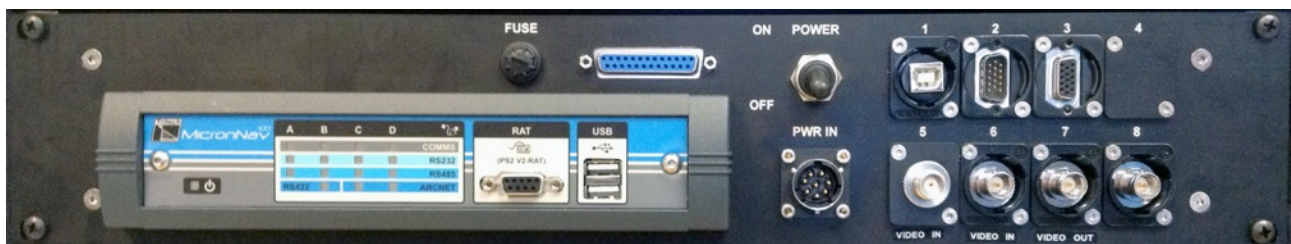
A typical SEU with MicronNav Hub installed
