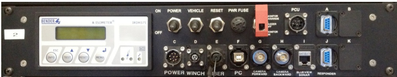
A typical fiber-optic SIU configuration
