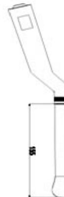
Figure 6-4. EC2-2/13R/6.5MHz Endo-vaginal probe protection against water ingress
