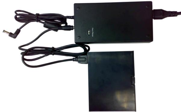
Figure 2-5. Charging through adaptive line
