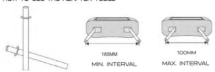
Since the spacing of the mounting holes can vary on different vehicles we supply two adapter poles {12mm diameter}, Use these adapter poles when the headrest mounting holes in your seat are too large for the posts of the headrest monitor.
