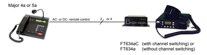
**Example 2:** Parallel circuit of several operation terminals --> LIM AC has to be equipped with notch for pilot tone.
