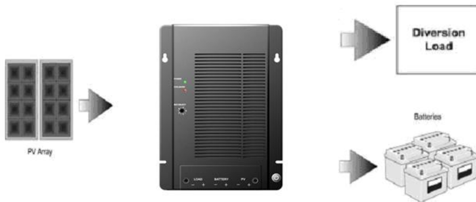
Figure 1-2: PV charge and load controller
