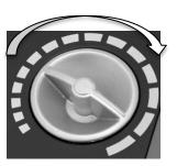
5. With the Heat Selector knob set to either "I" or "II", when the desired room temperature is reached, slowly turn the knob anti-clockwise until the heater turns off (you will hear a click).
