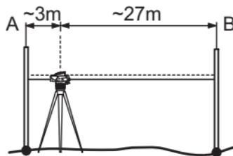
**Step 3:** Aim at Staff B and press MEAS key. Measurement display, press and hold measuring key for 3 seconds to accept.
