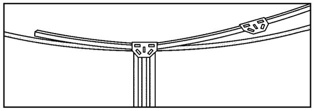
Insert the exposed end of a top rail into another top plate with a top rail inserted into the opposite side. Push the top plate with rails onto the edging again leaving the far end of the rail in the air. Continue in this manner all the way around the pool.
