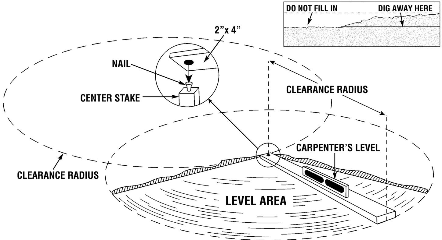
The assembled pool must have a vertical distance of 3' from the top of the pool to the adjoining grade and the adjoining grade must remain level for a distance of 4' away from the pool. Refer to the drawing at right.
