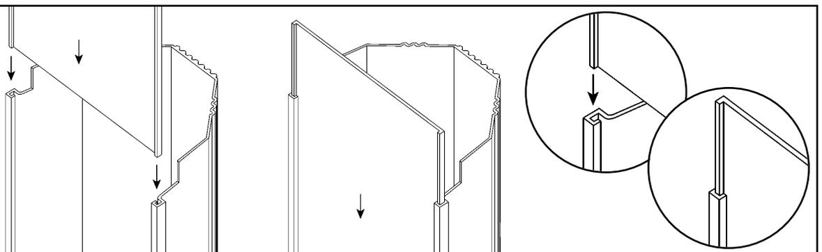
Insert two rails into a plate, in the same manner and using the same spacing as you have done on the bottom rail and plate assembly. Push the rails and plate assembly onto the plastic edging leaving the far end in the air.
