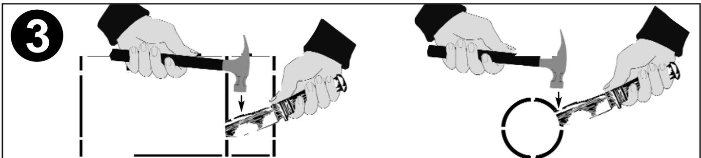
If the through wall filter inlet and outlet holes are to be used, remove metal cutouts by breaking perforations using a knife and hammer as shown. Refer to skimmer manufacturer's instructions for remainder of skimmer assembly. **Make sure skimmer does not leak as this will corrode the pool wall and cause a split in the wall that is not covered under the pool warranty.**
