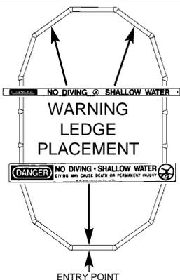
Your pool is equipped with (3) three special **warning** ledges. The (1) one ledge with a large **warning** on top is to be installed by the entry point into the pool and is not to be obstructed by any object such as your ladder. The (2) two ledges with the **warning** on the inside are to be placed opposite the entry point into the pool with the warning facing the entry point.
