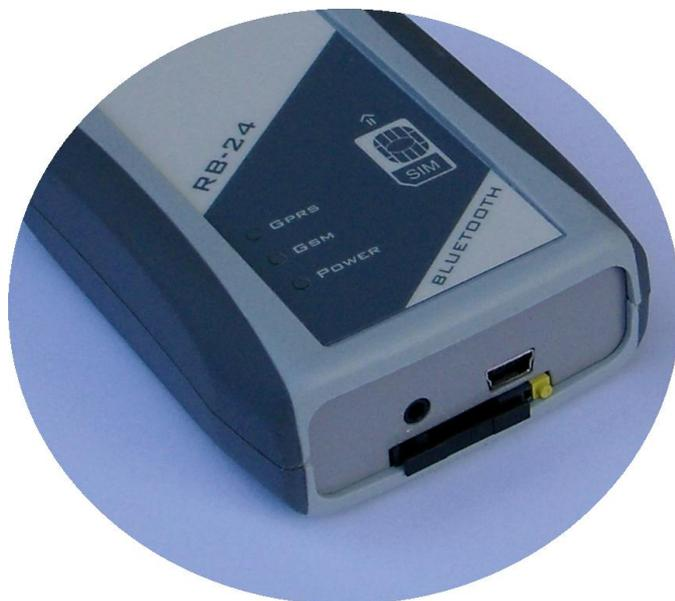
B) top panel: 3 LEDs state indicator: **POWER**, **GSM**(data), **GPRS**
