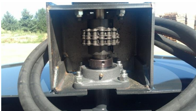
3.-4. Inspect chain and set screws-replace if necessary.
