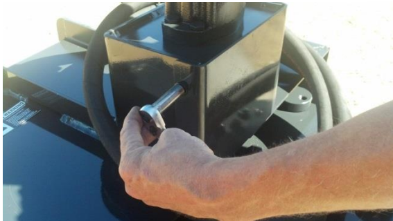
1. Remove Coupler Casing screws
