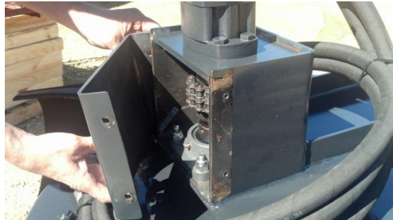
2. Remove Coupler Casing cover
