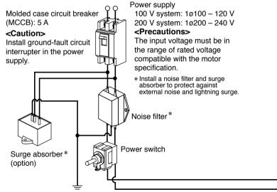
Ground the return circuit to the earth terminal. Should be class D earthing (100  $\Omega$  or less, ø1.6 mm or more).
