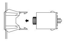
(3) Engage the hook with the base to fix it to the mounting frame.
