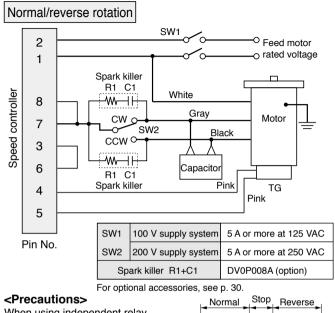
When using independent relay contacts for SW2 to change over normal/reverse, interlock both contacts so that they will not close simultaneously.
