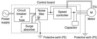
\* The length of connection cable between the speed controller and motor should be shorter than 3 m.
