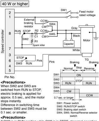
If SW2 is in RUN position while SW3 is in STOP, abnormal operation occurs (full speed rotation for a short time; or if SW3 is in RUN position while SW2 is in STOP, motor temperature rises excessively.
