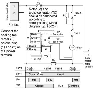
Once the TP operates, cooling period is required until the operation can start.
