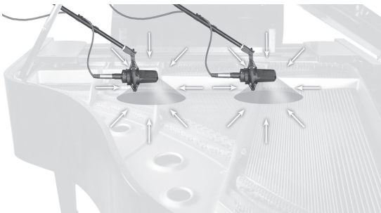
Figure 2. Conventional “Free Field” Microphones inside a piano only pick up sound accurately in front of the microphone
