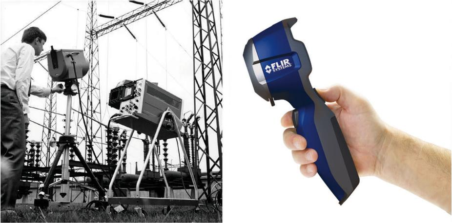
**Figure 18.2 LEFT:** Thermovision® Model 661 from 1969. The camera weighed approximately 25 kg (55 lb.), the oscilloscope 20 kg (44 lb.), and the tripod 15 kg (33 lb.). The operator also needed a 220 VAC generator set, and a 10 L (2.6 US gallon) jar with liquid nitrogen. To the left of the oscilloscope the Polaroid attachment (6 kg/13 lb.) can be seen. **RIGHT:** FLIR i7 from 2009. Weight: 0.34 kg (0.75 lb.), including the battery.
