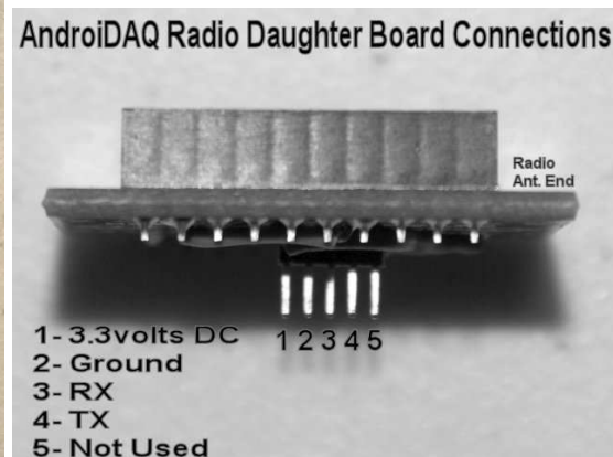
AndroiDAQ with Bare xBee foot-printed radio board and daughter board pin out numbers.
